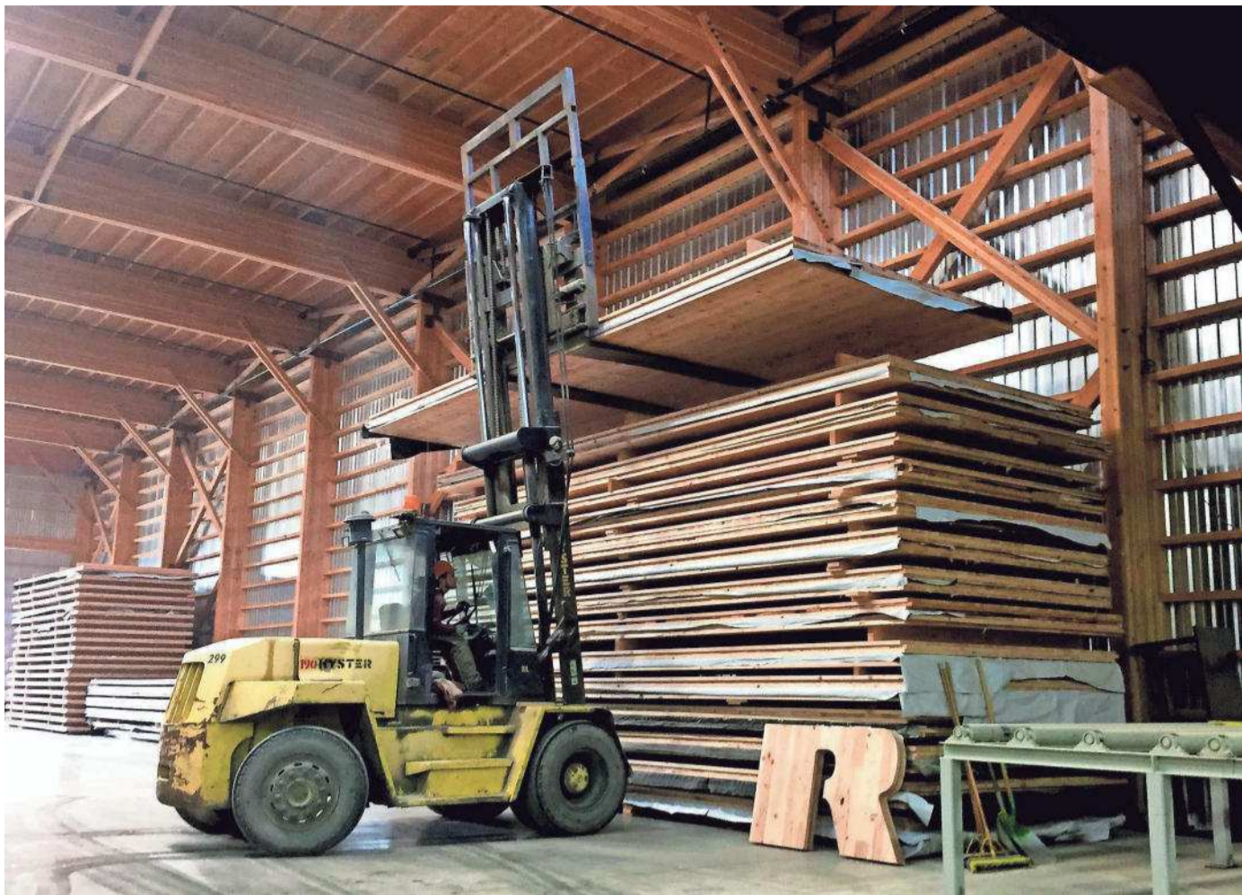
In this Nov. 11, 2016, photo, a forklift driver moves a newly assembled panel of cross-laminated timber, or CLT, to a stack in the production facility of D.R. Johnson Lumber Co., in Riddle, Ore. D.R. Johnson is one of just two companies in the United States currently able to produce CLT panels.
