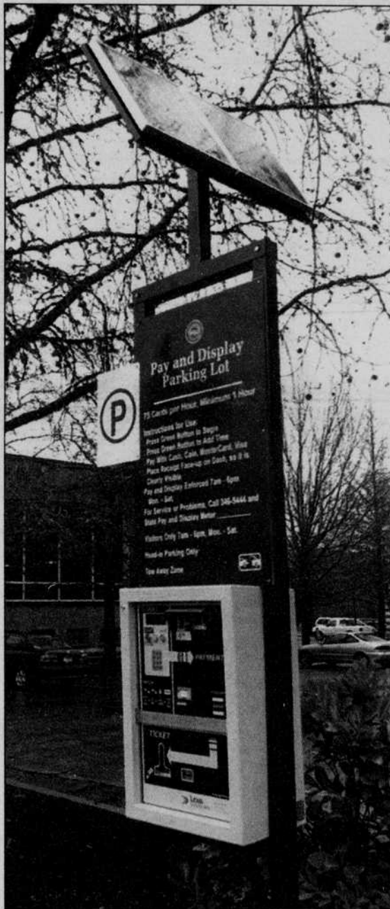
Environmentally friendly parking kiosks powered by attached solar panels, such as those now available in the EMU parking lot and in front of Oregon Hall, make parking easier by allowing drivers to use different payment methods.
