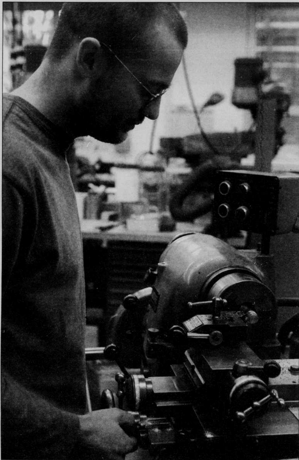
Machine shop supervisor John Boosinger demonstrates the Hardinge Lathe by reducing the diameter of a brass rod. The machine shop, located in the basement of Pacific Hall, is one of two shops operated by the Technical Science Administration that builds equipment.
