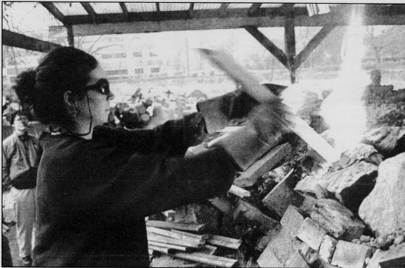
Allison Atwood stokes the 2,400 degree fires of an Anagama Kiln near the Millrace studios. The kiln, built by ceramics students, is patterned after a 7,000 year-old Chinese design and can hold over 1,000 ceramic pieces. Finished pieces will be on display at the Laverne Krause Gallery starting February 3 at 7 p.m.
