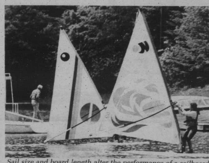
Sail size and board length alter the performance of a sailboard. Short boards move faster than long boards but are more difficult to control.
