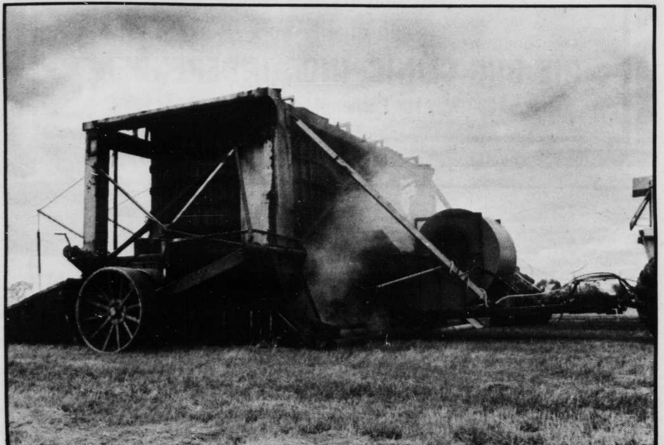
Experimental field burning machine in operation Tuesday near Eugene's Mahlon Sweet Airport. The 1971 Oregon Legislature stated that open field
