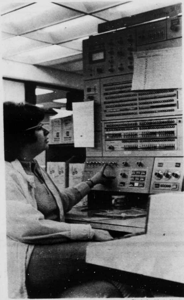
Photo by Linda Howe Linda Peterson works with an IBM 360-50 computer at the computer center on campus. At the center students can learn to develop techniques and programs for the use of computers and also can conduct research in statistics, numerical analysis and computer science.
