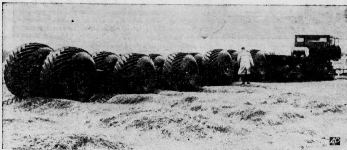
FIVE THOUSAND GALLONS of fuel are transported by this new carrier—a chain of 10-five-foot-high, 500 gallon capacity rubber tire bags. Advantage is rough terrain doesn't limit transportation. System was developed for Army's Transportation Research and Engineering Command by Four-Wheel Drive Auto Co., at Clintonville, Wis., and Goodyear Tire and Rubber Company.
