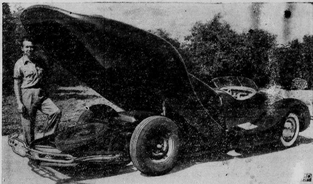
ULTRA-STREAMLINED AUTO — Norman E. Timbs, of Van Nuys, Calif., stands beside his car on which hydraulically-raised rear "deck" covers engine, gas tank and spare wheel.
