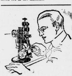
The holes for use in setting the lenses in eyeglasses or spectacle mountings are smoothly and accurately bored by this diamond drill.
