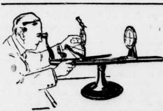
With this instrument the operator locates the optical center of the lens and also marks the axis of the cylinder, if any. It is also employed to check the accuracy of every completed pair of glasses. We call it the "policeman" of the shop.
