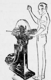
After the lenses have been cut to approximately the desired shape and size they are placed in one of these automatic edging machines and ground to accurate shape, with smooth even edges.
