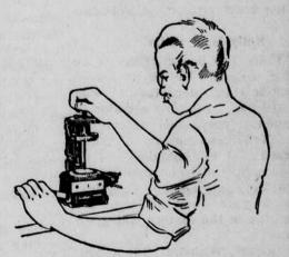
The holes for use in setting the lenses in eyeglasses or spectacle mountings are smoothly and accurately bored by this diamond drill.
