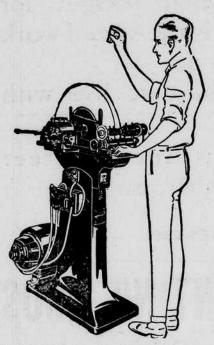
After the lenses have been cut to approximately the desired shape and size they are placed in one of these automatic edging machines and ground to accurate shape, with smooth, even edges.
