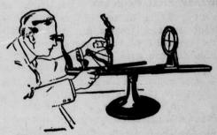
With this instrument the operator locates the optical center of the lens and also marks the axis of the cylinder, if any. It is also employed to check the accuracy of every completed pair of glasses. We call it the "policeman" of the shop.
