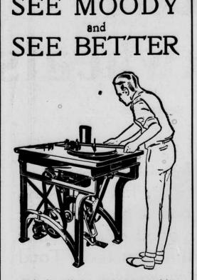
This is called a surfacing machine, and is used in grinding the surfaces of either flat or curved rough glass blanks to obtain in the finished lens the exact result required by your individual prescription. This operation requires careful, skilled workmanship
