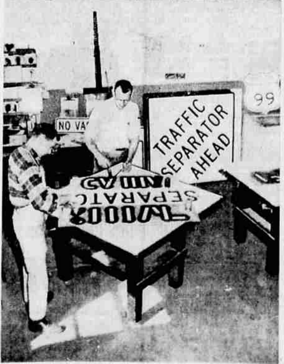
THE STENCILING ROOM in the Salem sign shop of the Oregon State Highway Department turns out a variety of work. Henry Hatfield, left, and John Helt work on a 48-by-48-foot traffic sign with black lettering on a light-colored reflectorized background. Signs are designed to give the greatest visibility, day or night. (Oregon State Highway Department photo)
