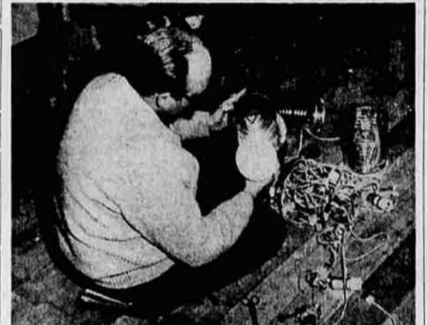
INGENUITY plays a major role when it comes to constructing and equipping a theater with limited funds. Allen Nash is shown here fitting tin cans as reflectors and covers for special lights.
