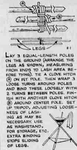
LAY 3 EQUAL-LENGTH POLES ON THE GROUND (ARRANGE THE LEGS AS SHOWN), MEASURING FROM ENDS TO LASH AREA BEFORE TYPING. TIE A CLOVE HITCH ON SET POLE. THEN WRAP 3 LOOSE TURNS AROUND POLES AND BIND THESE LOOSELY WITH 2 TURNS BETWEEN POLES. FINISH WITH ANOTHER CLOVE HITCH AROUND CENTER POLE. SET UP TRIPOD, ADJUSTING LOOSENESS OF LASHING AS MAY BE NECESSARY. USE AS WASHSTAND, FOR STORAGE, ETC. EXTRA BINDING: STOP SLIDING OF LEGS.
