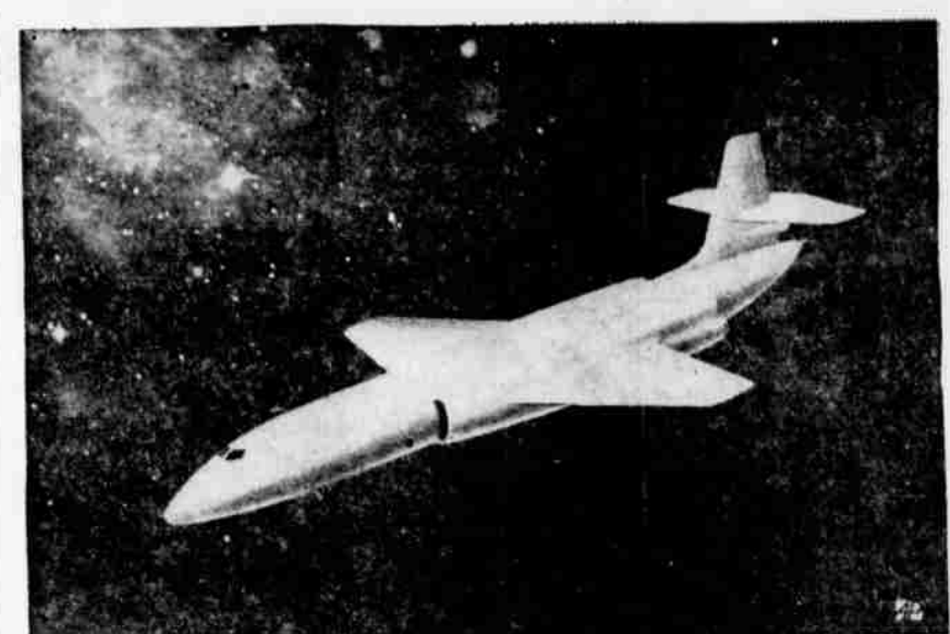
U. S. ATOMIC BOMBER — This is an artist's conception of a possible American atomic bomber. It has not been built or even started. This sketch was prepared last year by Lockheed Aircraft Corp., which is working on the overall design of a possible U. S. A. plane. In this American conception there is a single nuclear engine in the body of the plane, just behind the wing. The turbojet air intake is in front of the wing. Crew compartment is up front so as to keep the men as far away from the radioactive reactor as possible. (AP Wirephoto)
