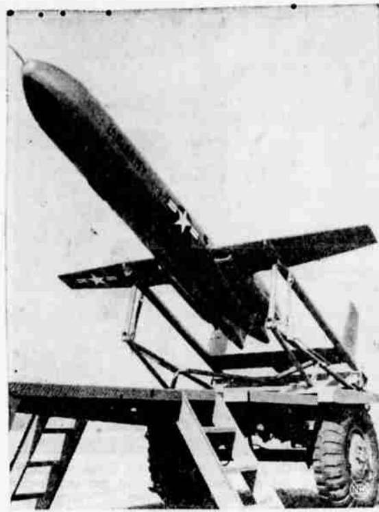
SKY SPY —An air-to-ground robot "spy," the Republic SD-3 combat surveillance drone is shown above on its portable launching platform. Currently undergoing flight tests with the Army Signal Corps, the pilotless drone switches from television to radar, infra-red or photographic sensing devices by means of interchangeable nose units. Driven by a pusher propeller, it is launched initially by JATO rockets.
