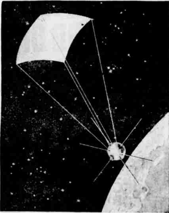
SOLAR SAILS IN THE SUNSET —Space travelers of tomorrow may well be "sailors." One scientist has proposed the use of "radiation pressure" sails as a means of getting around the problem of transporting bulky and heavy chemical fuels on long space journeys. Drawing above pictures this idea, the branch chief of General Electric engineer Norman F. Barnes. A thin plastic sheet, attached to a satellite or spaceship, utilizes the small but steady force of particles of light called "photons" which continually stream from the sun at 186,000 miles a second. Striking the sail, these particles exert a force that could, according to Barnes, increase the space vehicle's speed by about 250 m.p.h. each day.
