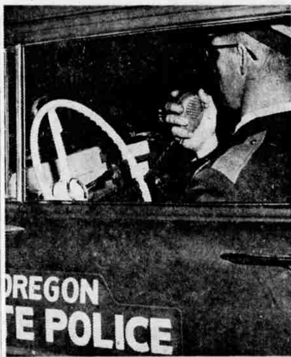
SPEED WATCH — Officer Wright, private first class of the Oregon State Police, watches the dial of his radar-equipped car for speeders. When one is noted, he radios ahead to another officer who halts the offender.
