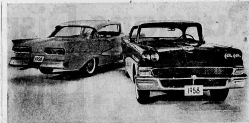
STYLING CHANGES in the 1958 Ford line are apparent in these views of the Fairlane 500 Town Victoria, right, and Fairlane Club Victoria, left. Dual headlights, corrosion-proof aluminum grille, inverted-V trunk lid and new taillight design are among the changes. Ford offers new engines, automatic transmission and air suspension. The new Fords are on display today at Lockwood Motors, 721 SE Oak Ave.
