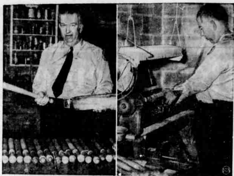
HOBBY WITH A WALLOP —Many a headache for the woodworker has come from the backyard woodworking shop of H. O. Harper, a Columbia, S.C., policeman. He turns out night sticks, those handsome shillalaha which are the patrolman's symbol of authority. At left, he displays a piece of stovewood from which he fashions the persuaders on his lathe at right. He uses hickory or oak. Most of the Columbia force carries his sticks and many have gone to colleagues in other cities.
