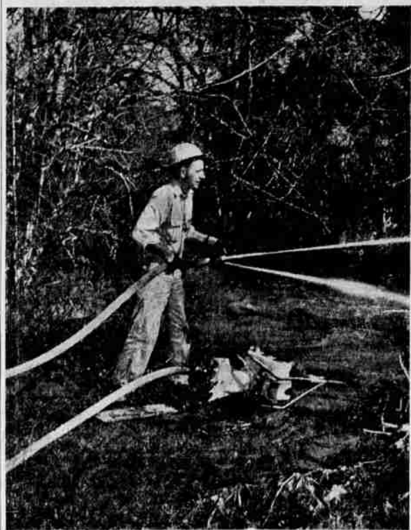
POWERSAW FIRE ENGINE —Cecil Cunningham, assistant forester at Weyerhaeuser Timber Company's branch in Springfield, Ore., is pictured above demonstrating a powersaw converted into a portable fire engine for fighting forest fires. Company foresters at Springfield invented attachments by which a powersaw may be converted to fire fighting purpose within 90 seconds.
