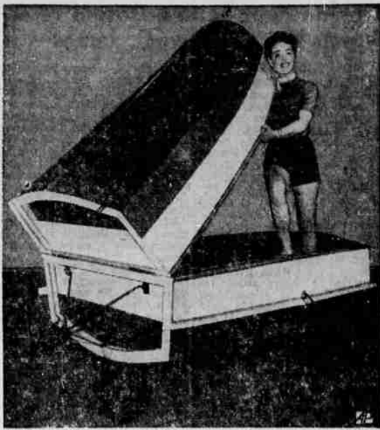
EASY TO LAUNCH —Terry Georgian demonstrates how simply this trailer boat, exhibited at Chicago National Boat Show, is made ready for use. Body unfolds and wheels are removed.
