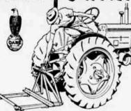
Speed your chores with tractor power! Case Utility Carrier hooks up in a minute, right from tractor seat. Lifts and carries all those awkward loads too heavy for a man, too small to need a wagon. Lowers for easy loading, raises with
