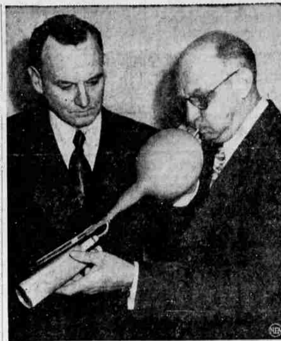
"NOW, SHEE HERE, OFFISHER!" — Driving drunks won't stand a chance when confronted with this little chemical gadget, "The Drunk-o-meter." The gadget, shown at a traffic conference at the University of Washington, Seattle, measures the alcoholic content of a man's breath. Anything over 15 per cent means he's "under the influence." Dr. C. W. Muehlberger of the Michigan State Department of Health tests the "intoximeter," while Theodore Loveless of the University of Washington looks on.
