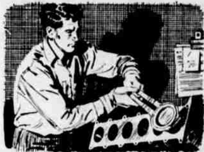
1. New atomic tool! Our scientists equipped test engines with piston rings treated at the Atomic Energy Commission's Oak Ridge Plant. For the first time, science measured wear as it happened!
