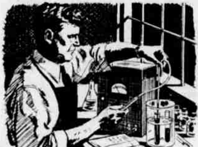
2. Geiger counters detected the rate at which metal wore away from these atomically treated rings—under different circumstances, and with different oils!
