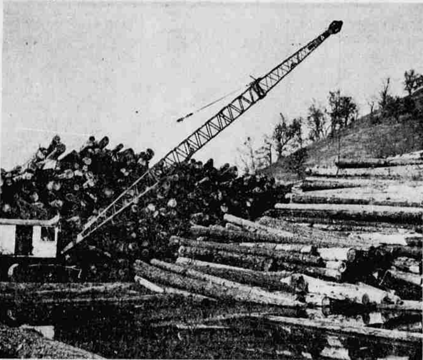
PICTURED HERE is a huge crane in use by the Roseburg Lumber company to cold deck logs at its Dillard mill. These logs have been hauled to the pond by truck, dumped and floated to the crane set by men with pike poles, calked boots and fine sense of balance. The logs are ricked in decks 20 to 30 feet high, where they will remain until needed for sawing. The logs used at this mill are fir and are representative in size of those used by the industry in this locality. —(Story and picture by Paul Jenkins).
