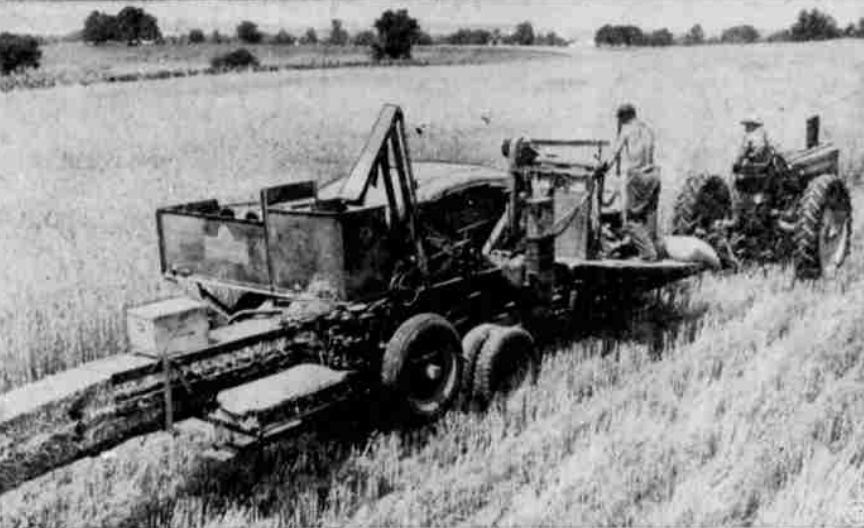
COMBINES COMBINE —Martin S. Zimmerman, New Holland, Pa., farmer, is a man in a hurry when it comes to harvesting his big wheat crop. So he fixed up the unusual machine, above, by joining a standard automatic baler and a combine to make one machine that does several jobs. Here a two-man crew is cutting the ripe wheat, threshing it to separate chaf from grain, bagging the grain and baling the left-over wheat straw in one continuous operation. At left, an automatically twine-tied bale is ready to drop from the baling chamber.
