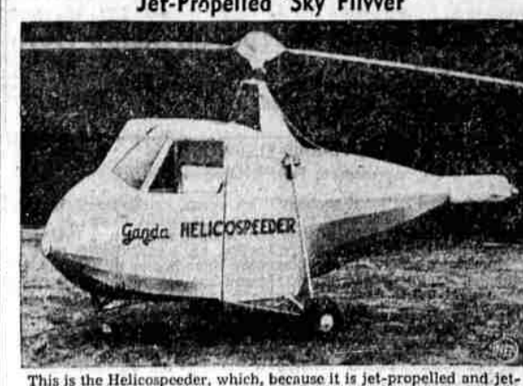
This is the Helicopter, which, because it is jet-propelled and jet-steered, is said to have more speed, carries more weight, has more stability and controllability than an ordinary helicopter. Invented by Antoine Ganga, of New York, the craft omits the auxiliary tail rotor common to the usual helicopter.
