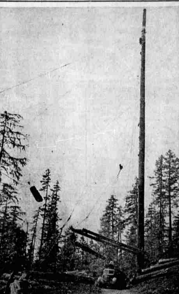
A "HAYRACK" loading boom in extremely rough country high on the shoulders of Mt. Scott, in the logging woods of the Roseburg Lumber company.
