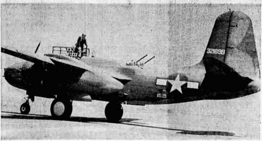
A power turret housing two .50-caliber machine guns is the latest addition to heavy fire power of this deadly Douglas A-20 Havoc bomber just off the assembly line at Douglas' Santa Monica, Cal., plant. The Army reveals that the famed bomber now packs nine .50-caliber guns.
