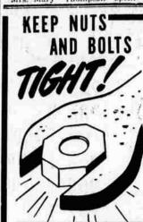
\* Loose nuts and bolts invite wear and breakage. It's good practice to inspect the m carefully during service periods.
