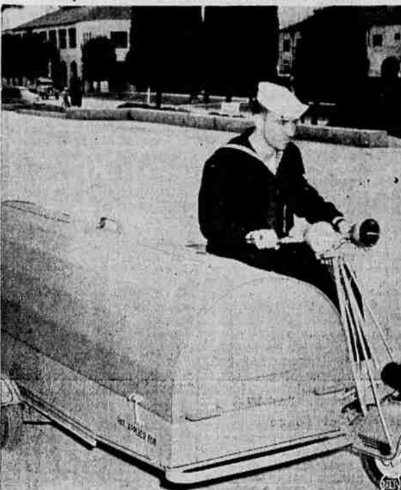
The latest in motorized hospital equipment, a "putt-putt" ambulance, is what R. L. Walker, pharmacist, third class, used to transport injured or ill recruits to San Diego's naval training station. It weighs 425 pounds and can travel 35 miles an hour.
