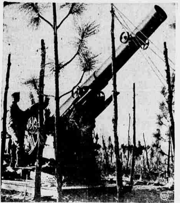
Big gun ringed by camouflage framework for action in First Army's South Carolina maneuvers is 240 mm. howitzer, largest U. S. field artillery weapon. It throws a 345-pound shell nearly five miles high to a distance of more than nine miles. The howitzer is manned by crew from 29th Field Artillery, so far the Army's only regiment equipped with this powerful gun.
