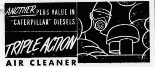
Tractors... like the human body... keep healthier if they breathe clean air. The air used by "Caterpillar" Diesels is triple-cleaned; first, at the inlet screen; next, in a whirlwind action; and finally in a bath of oil.
