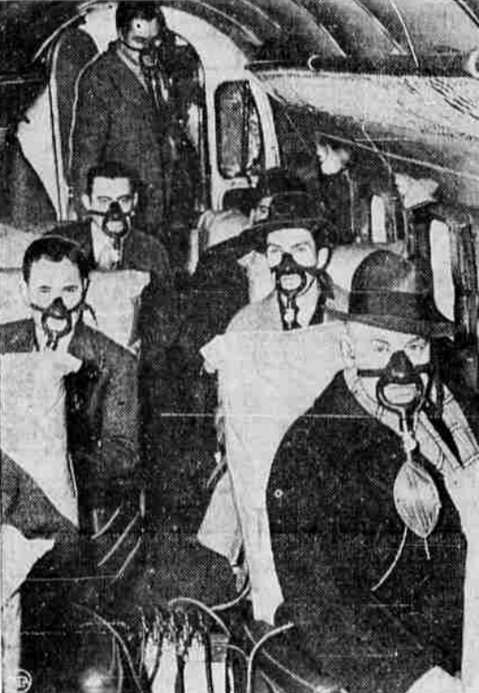
Gas masks for peacetime. Ten passengers breathe mixture of helium and oxygen in successful test of sub-stratosphere passenger flying 20,000 feet above Minneapolis, Minn. Outside this Northwest Airlines plane, the temperature was 32 below.
