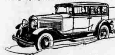
The Roosevelt—Roomy, sturdy, economical to operate. 30 horsepower, Marmon-built straight-eight motor.
