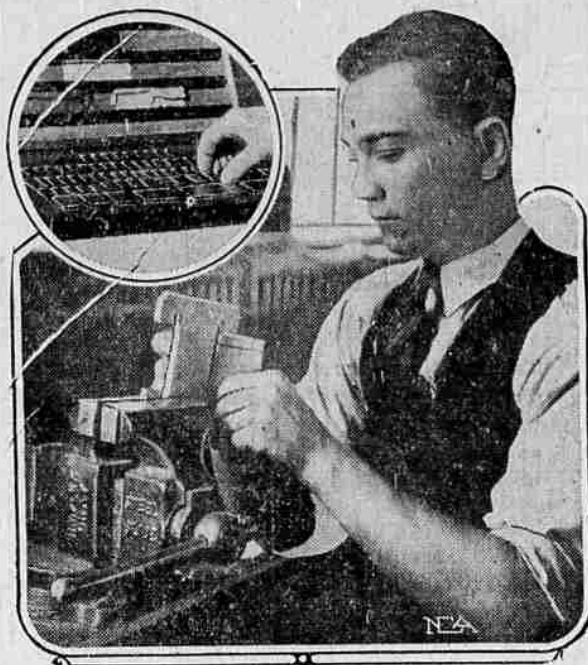
Lapping a snap-gauge, shown here, is work requiring skill and ex- treme care, for there's only one ten-thousandth of an inch difference between the jaw widths. Inset shows a set of Johansson guages, the standard of all.
