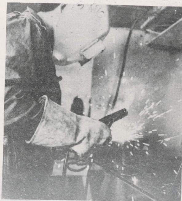
Denny Akeya demonstrates his skill in using the electric arc welding machine in the fabrication of the go-cart frames as he joins metals.
