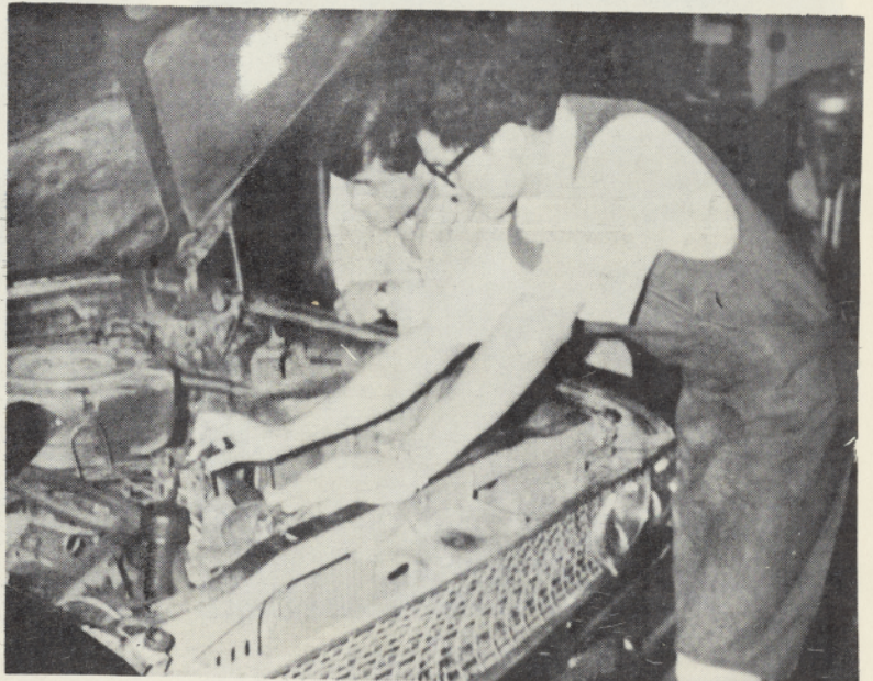
Alfred Kasuse and Frank Etcitty are setting the timing on an automobile engine. This is just one of the many phases of automobile repair.
