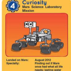
needs: lasting water and the right chemical ingredients. Weight: 1,982 lbs Top Speed: 0.09 mph Toolkit: 10 science instruments
