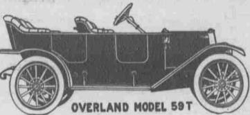
Wheel base 166 inches; motor 4x4%; horsepower, 30; Splitdorf magneto; transmission, selective, three peeds and reverse; F. & S. ball behrings; tires, 32x3%, Q. D.; 3 oil lamps and generator; complete out-tit, top, top hood, windshield and spedometer,
