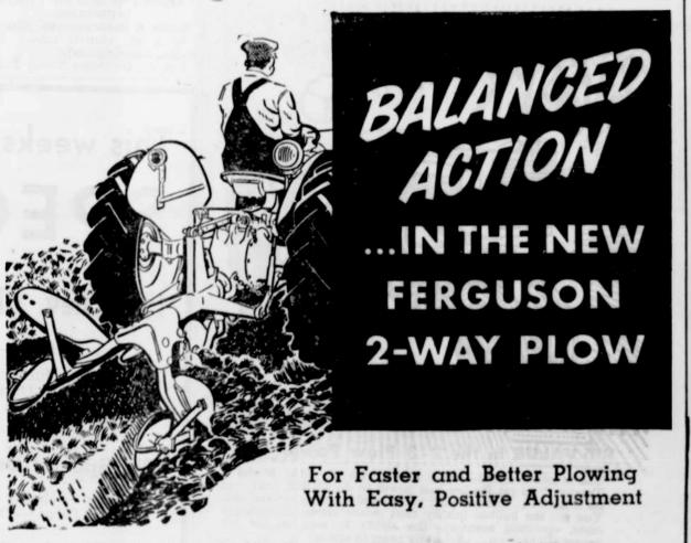
Balanced action in this New Ferguson 2-Way Single-Bottom Moldboard Plow speeds up seedbed preparation. Gives quicker entry and faster turnarounds at the headland. Operates efficiently at all plowing depths up to 12 inches. Big 18-inch base covers heavy trash, or green manure crops. This new 2-way plow is tractor mounted with fast three-point attachment. Each base has own coulter-jointer combination. Exclusive
