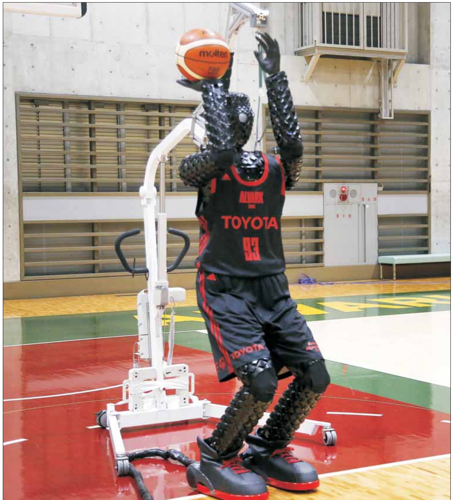
THREE-POINT THREAT. Toyota's basketball robot, Cue 3, takes a shot at a gymnasium in Fuchu, Tokyo. The 6'10" machine made five of eight three-pointers during a demonstration in a Tokyo suburb, a ratio its engineers say is worse than usual. Toyota Motor Corp.'s robot computes as a three-dimensional image where the basket is, using sensors on its torso, and adjusts motors inside its arm and knees to give the shot the right angle and propulsion for a swish. See story on page 8. (AP Photo/Yuri Kageyama)
