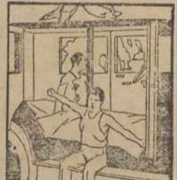
Both seats and upholstery make into a full sized bed in the car for camping.
