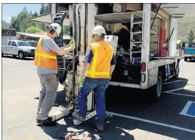
Contractors use a small drilling rig to collect groundwater samples near Canyon Boulevard in southwest John Day.
