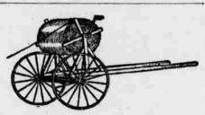
it from unwinding too rapidly. For winding up wire the machine is best pushed just fast enough to keep up with the wire as it is being wound on the reel. A crank placed upon the reel proves serviceable in winding up. -Farm and Home.
