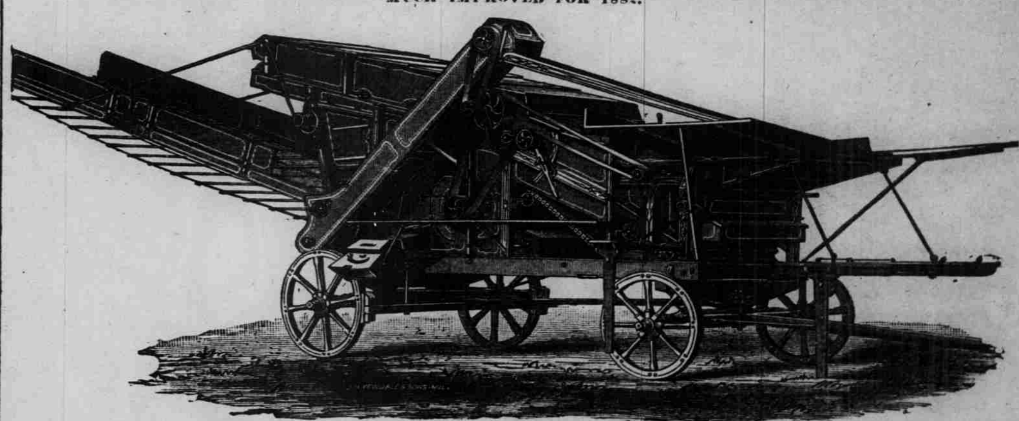
Has Long Straw Rake. Separates Cleaner from Straw than long apron and Short Straw Rake. It has the short, quick end Shave on Shoe. Never Clogs in Tar weed or Fern and does not throw grain over. Less Hops. The drive belt passes around the beater and Fan Pulley and is provided with a lighter Square gear substituted for the troublesome cross belt. Cranks less grain. Runs lighter and threshes faster than any machine in America.
