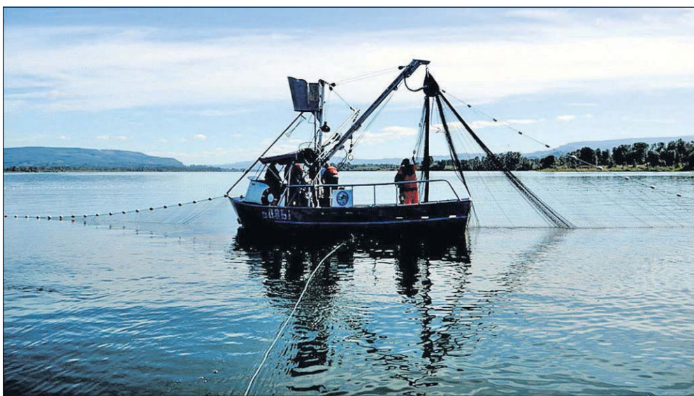
Washington Department of Fish and Wildlife A small purse seine is deployed on the Lower Columbia River. The net is played out in a large circle, ready to be drawn or "pursed" in. Theoretically, any fish caught within the purse can be sorted through, with wild-spawning individuals released back into the water, while hatchery fish are retained.
