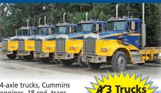
engines, 18-spd. trans. (RTLO18918B), single spd. Eaton rear-ends (DS462P). 4:11 gears w/locker. Hendrickson Haul-Max
